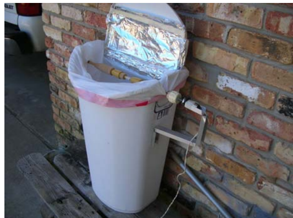
Fig 04 A Containment System Compressed Air Spraying
